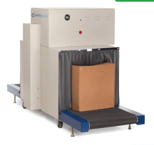
The rugged 10080T is designed to screen large items for potentially hidden explosives, weapons, narcotics and other contraband. Whether searching for threats in large boxes, cargo or checked baggage, this powerful unit delivers clear, sharp images. The system's 160 kV rated generator and multi-energy color marking enables operators to rapidly and easily spot organic, inorganic and mixed materials in even the most crowded boxes or bags.
