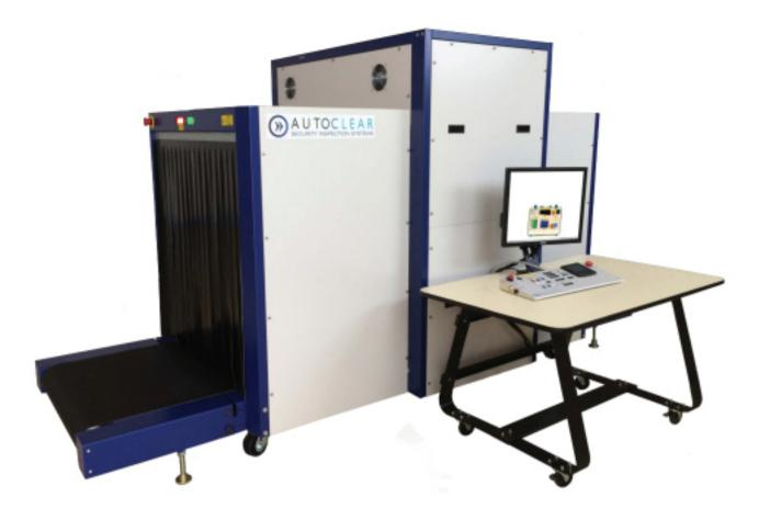
The 100100TDVS heavy-duty conveyorized X-ray inspection system is designed for screening large objects, hold baggage and cargo for concealed weapons, explosives and contraband. Multi-energy color allows operators to quickly spot areas of concern in the most thickly packed parcels, bulk loads and baggage. The system's high-capacity conveyor sits less than a foot from the floor for easier, more ergonomic loading.
